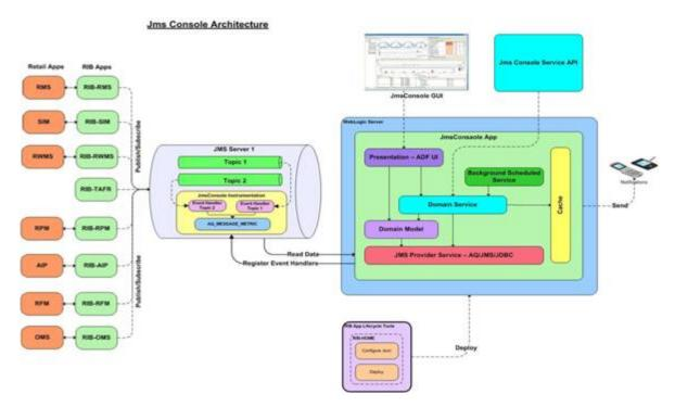
The AQ JMS that the application is monitoring is configured as a JDBC data source in the application server. The application dynamically discovers the topics and subscribers configured in the AQ. The application interfaces with the AQ JMS using PL/SQL API's provided by the AQ and uses instrumentation techniques to collect statistics using PL/SQL procedures.
